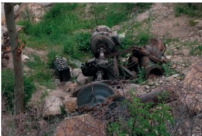
Picture 2.14: The MHPS in Rijist is a patchwork of old equipment (water pump, truck axis and generator), and is not even fixed on the ground. (Photo: T. Hoeck, June 2003)
