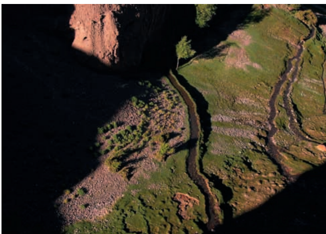
Picture 2.42: Water supply in Savnob depends on a single spring feeding water channel for irrigation, hydropower and drinking water. (Photo: T. Hoeck, June 2003)
